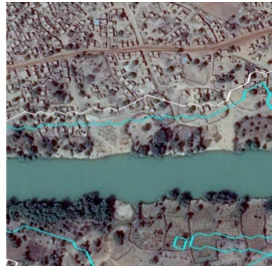
Figure 4. The Sirba flood line at Tallé according a 100 years (white) and a 20 years (light blue) return period.
