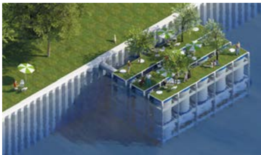
Figure 2. LURITEC installation in a river or lake as an element of integrated town planning. Source: LURI.watersystems. GmbH.
